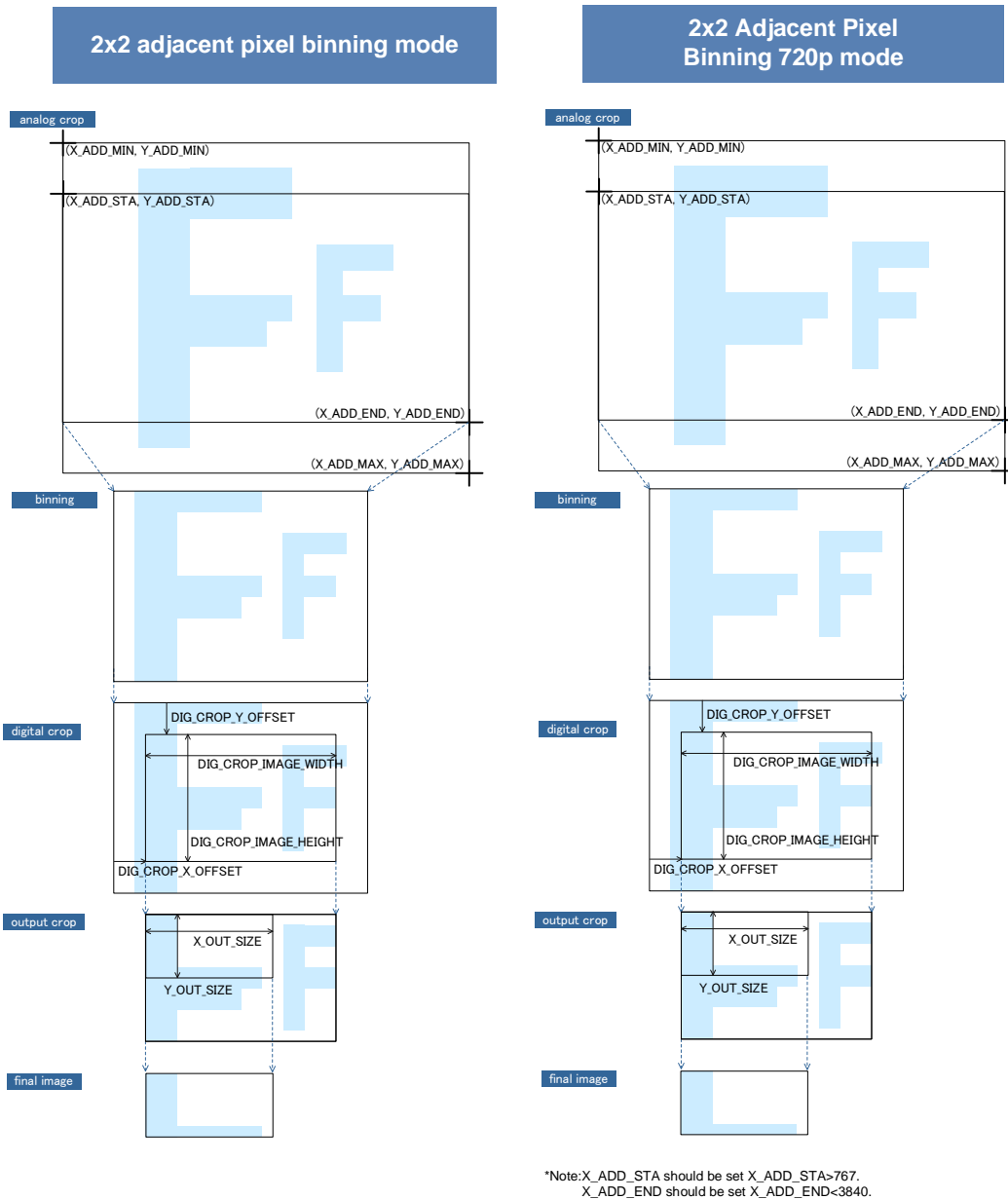
Figure 15 image area control capabilities for 2x2 adjacent pixel binning mode and QBC HDR mode
